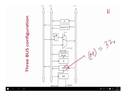
Let us assume that the memory location M has the value of 32 let us assume this. So, now, the MDR has the value of 32. Now we have two write it to basically register R\_1. So, this step is more simpler in a single bus architecture, let us assume that we have a single bus architecture here and we have only C, let us assume that only C is available and 32 is available over here.
