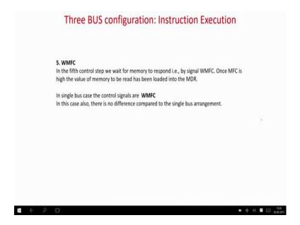
So, now the memory address register will have the value of M. Now we have to wait for some amount of time till the memory is ready, then the value will come to memory data register in fact, that was also similar for the single bus architecture.
